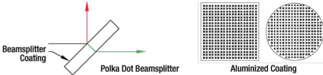
Polka dot beamsplitters are useful over a wide wavelength range and are negligibly angle sensitive, which makes them ideal for splitting the energy emitted from a radiant source. These are not recommended for imaging applications, such as interferometry, as the polka dot pattern will affect the image.
