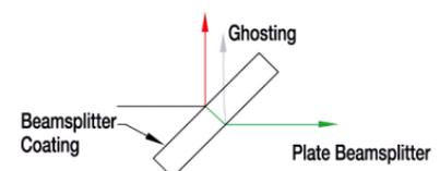
**Economy Beamsplitters** - These are the most cost effective of all the beamsplitter types. Thorlabs' economy beamsplitters, which have an exposed oxide coating on one side and are uncoated on the
