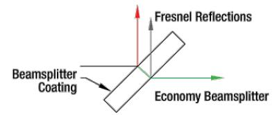
Please note that the Fresnel reflections off of the uncoated back surface of these economy beamsplitters can lead to interference effects in the reflected beam. For applications sensitive to these effects, consider using a beamsplitting cube or a pellicle beamsplitter.
