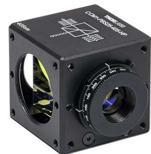
Click to Enlarge Figure 3. Screw the rotation mount onto the SM1-threaded input aperture of the mounted beamsplitter cube to complete the variable attenuator.
