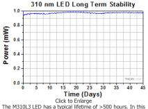
Click to Enlarge The M310L3 LED has a typical lifetime of >500 hours. In this case, the unit under test continued to provide more than 95% of its initial power after 45 days.
