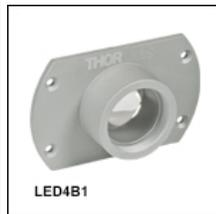
The LED4B1 Adapter for Liquid Light Guides contains a collimating aspheric lens (Item # ACL2520-A) to focus light from the 4-wavelength LED source into a liquid light guide (LLG) held in the appropriate LLG-to-SM1 adapter (not included). We manufacture two of these adapters: the AD3LLG SM1 adapter for Ø3 mm core LLGs and the AD5LLG SM1 adapter for Ø5 mm core LLGs. Thorlabs' selection of liquid light guides can be found [here](#).
