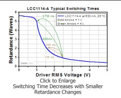
In addition, the material's viscosity and hence the switching speed also depend on temperature of the LC material. As can be seen below, the switching speed can increase by as much as two times by heating the LC retarder. Our standard LC retarders are designed to work at temperatures of up to 45 °C, where they can still maintain the specified retardation. If additional speed is required, the retarders can work at temperatures up to 70 °C, but the maximum retardation value will be lower.
