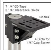
C1505 fits any Ø1.5" diameter post. The angle bracket provides an array of mounting options including seven 1/4"-20 (M6) mounting holes, two 1/4" (M6) clearance holes, and four 1/4" (M6) clearance slots. Once the platform height has been established the post clamping mechanism is actuated with a 3/16" (5 mm) hex key or balldriver.
