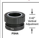
The PSHA Adjustable Height P-Post Collar offers a convenient height adjustment for post mounted hardware. An easy-to-access actuator ring allows fine height adjustment at 0.025" (0.64 mm) per revolution. The photo to the right shows the PSHA on a Ø1.5" Post below the C1505 Mounting Post Bracket (sold above).
