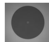
Click to Enlarge Undamaged Fiber End
