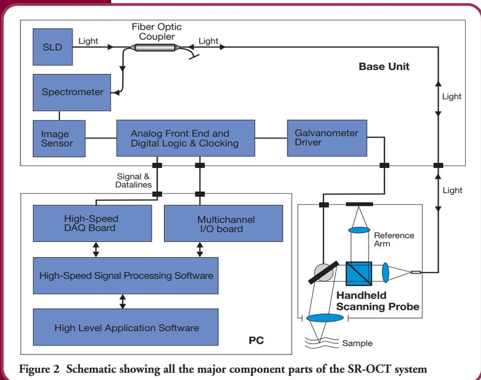
Figure 2 Schematic showing all the major component parts of the SR-OCT system
