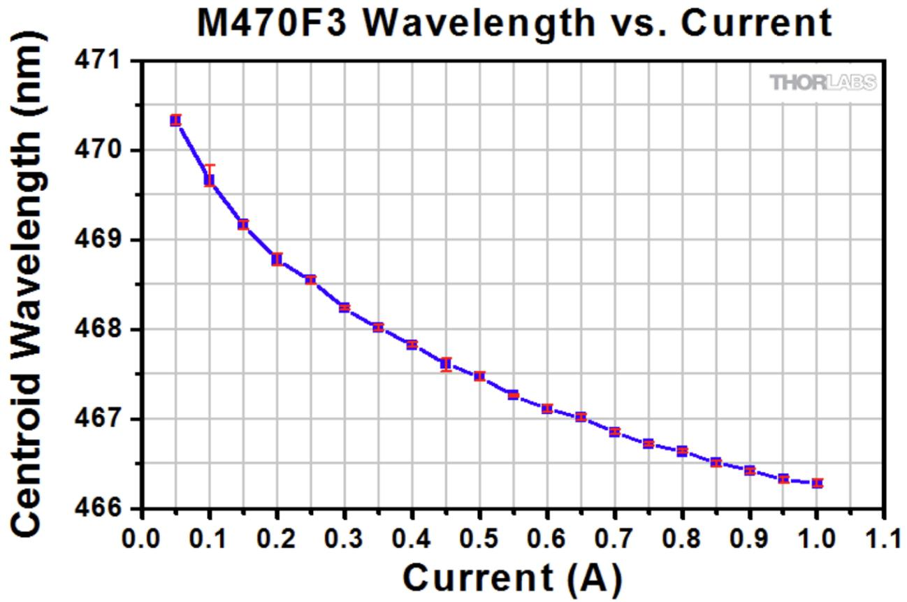
A graph of the centroid wavelength measured at different drive currents. Four sets of measurements were taken. Each blue square represents the average centroid wavelength across all runs for a given current. The minimum and maximum measurements at each current are represented by the red error bars.
