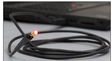
Click to Enlarge Figure 4.1 A LED630L being powered by the USB port in a laptop.
