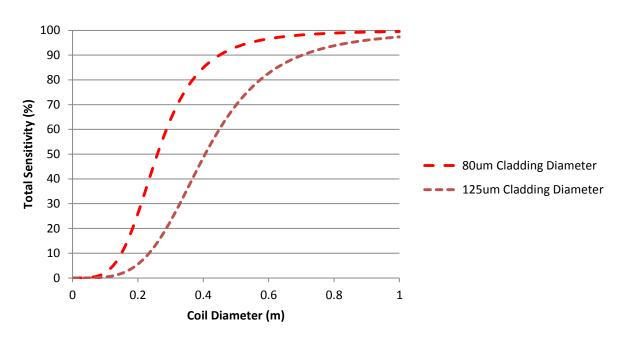
Figure 4: Spun LoBi fiber sensitivity variation with coil diameter and cladding diameter.
