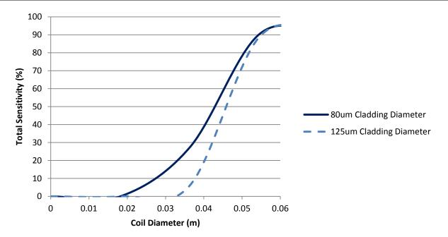
Figure 5: Spun HiBi fiber sensitivity variation with coil diameter and cladding diameter.
