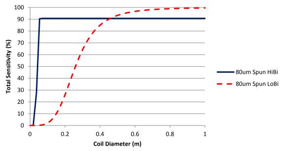
*Figure 3:* Theoretical comparison of the sensitivities achieved using an 80µm cladding diameter spun HiBi fiber and an 80µm cladding diameter spun LoBi fiber.
