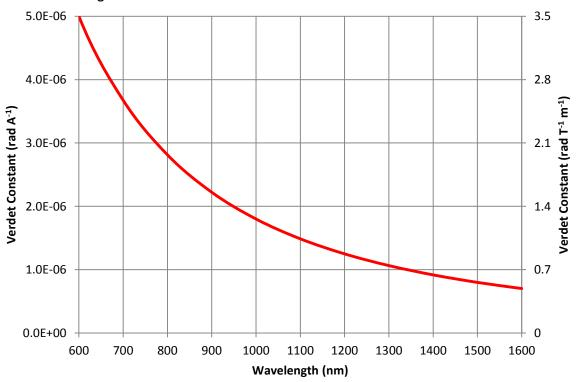
Figure 2: Variation in Verdet constant with wavelength for a silica core fiber [2].
