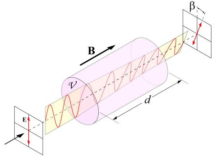
**Figure 1:** Polarization rotation as linearly polarized light passes through a material with a Verdet constant, V, and a distance, d. The polarization rotation,  $\beta$ , is proportional to the magnetic field, B.[1]
