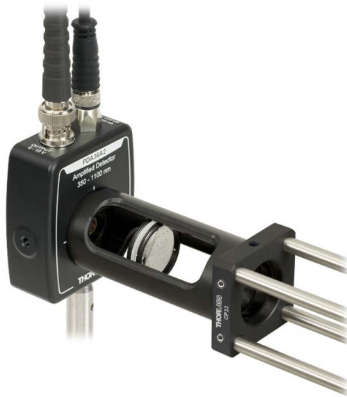
PDA series photodetector mounted onto a Ø1" Slotted Lens Tube, which is housing a focusing optic. The lens tube is attached to a 30 mm cage system via a CP33 SM1-Threaded 30 mm Cage Plate. This arrangement allows easy access for optic adjustment and signal alignment.
