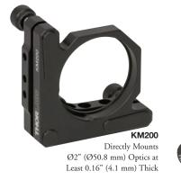
The KM100 and KM200 are our most popular mirror mounts. The models feature brass bushings, high-quality 1/4"-80 adjuster screws, and hardened inserts at key wear points. The stability of these mounts is achieved using thick front and back plates, which support strong springs and enhance performance. For your convenience, these mirrors are stocked for same-day shipment with broadband dielectric mirrors.
